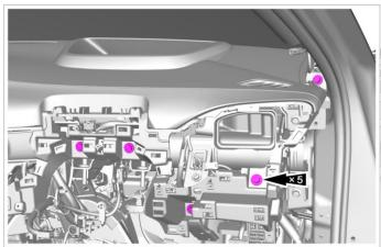
11. Remove 3 fixing bolts in the middle of instrument panel upper body assembly.
