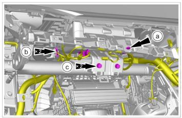
17.18. Disconnect 4 connectors from the instrument panel upper body assembly.
