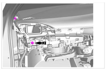
14. Disconnect 1 connector from the right channel temperature sensor assembly of instrument panel upp er body assembly.
