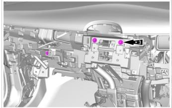
12.13. Remove 2 fixing bolts on the left side of instrument panel upper body assembly.
