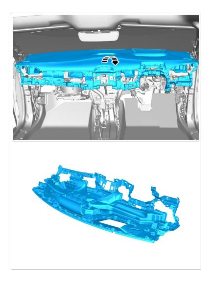
$20. \ \ To\ replace\ the\ instrument\ panel\ upper\ body\ assembly,\ remove\ the\ following\ accessories\ from\ it:$
