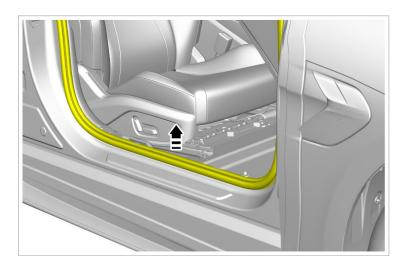
2. Remove 1 plastic nut from the right A-pillar lower shield assembly.
