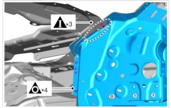
9. Remove 18 welding spots and take out the right A-pillar inner panel assembly.
