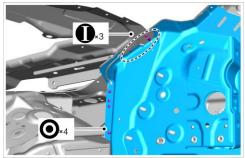
Weld 14 welding spots on the right A-pillar inner panel assembly.
