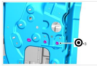
7. 8. Weld 18 welding spots on the right A-pillar inner panel assembly.
