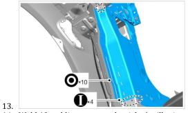
14. Weld 10 welding spots on the right A-pillar inner panel assembly.
