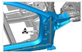
12.13. Remove 11 welding spots of the right side wall assembly.
