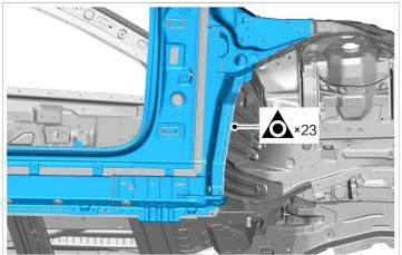
16. Remove 50 welding spots of the right side wall assembly.
