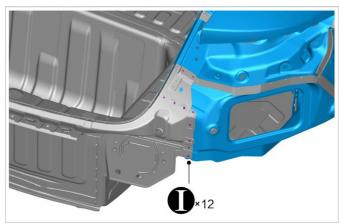
Weld 15 welding spots on the right side wall assembly.
