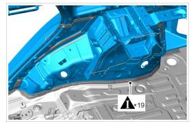
Remove 19 welding spots of the right side wall assembly.
