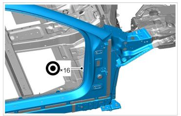
18.19. Weld 19 welding spots on the right side wall assembly.
