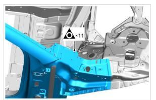
14.15. Remove 23 welding spots of the right side wall assembly.
