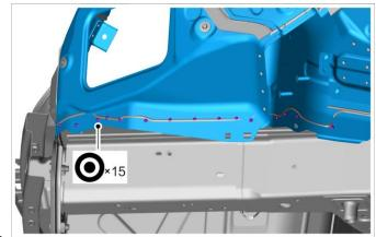
10.11. Weld 50 welding spots on the right side wall assembly.
